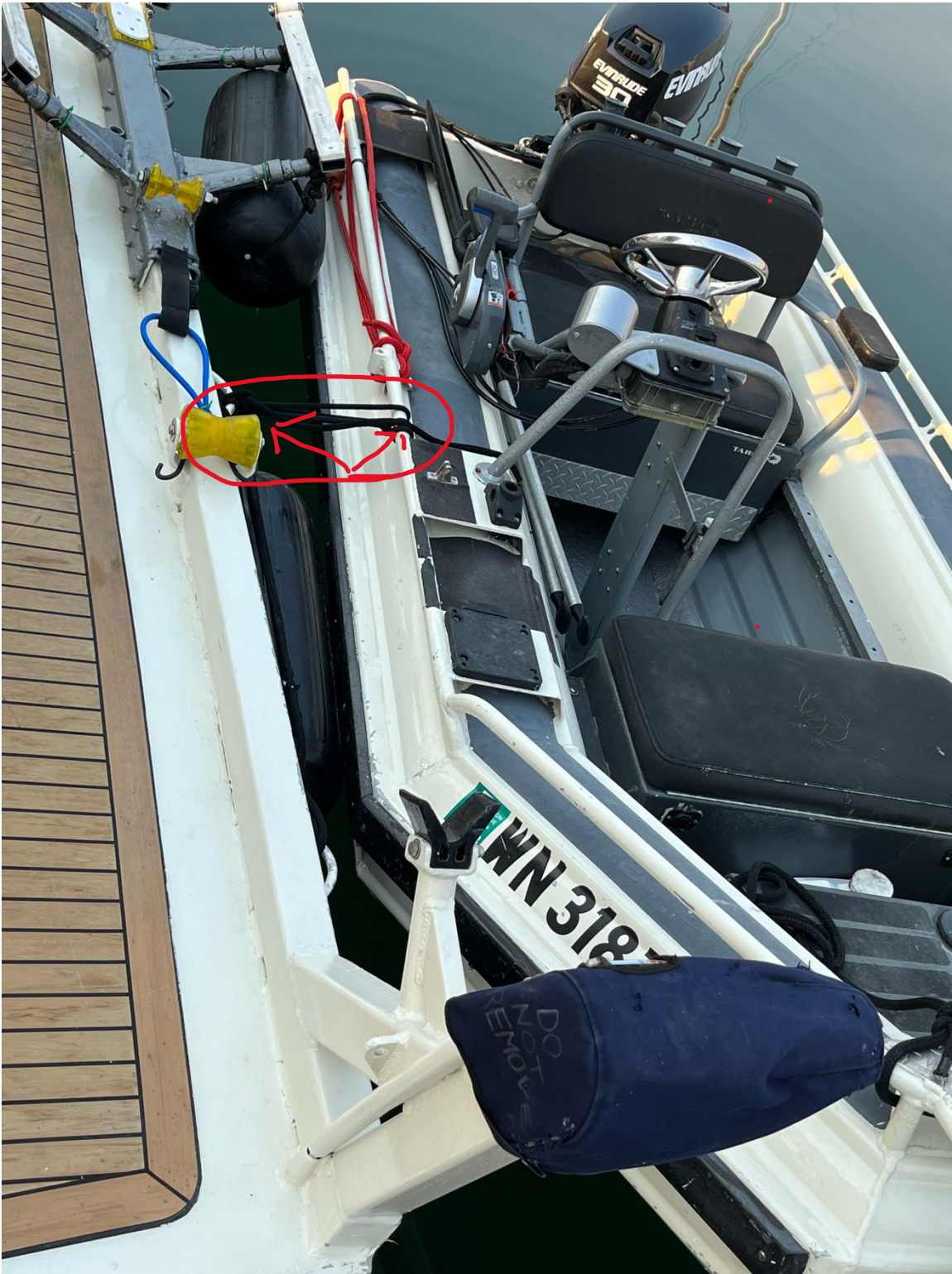
Proper tender tie-off to stern when boarding.
