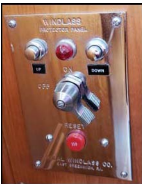
The windlass breaker is to right of the lower helm.
