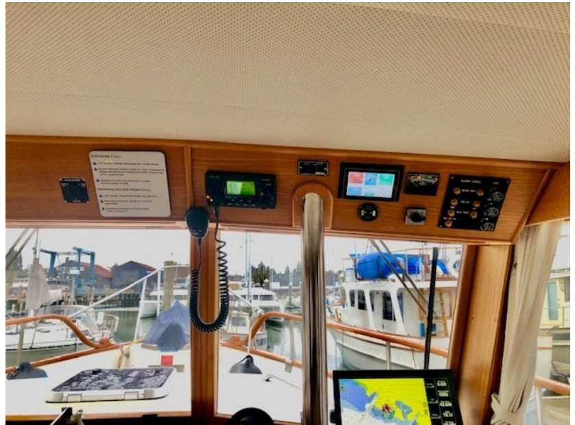
Lower Helm, Chartplotter, VHF, Inverter Display, Safety Panel
