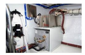
There are three sources of heat on True Blue: Hydronic Diesel Furnace, and 2 - 120v electric.
