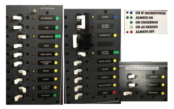
When not connected to shore power or when using the generator as an A/C source, the batteries are providing all power. Therefore, monitor the use of onboard electricity carefully with your volt meter located on the DC Panel, and turn off electrical devices that are not needed. Note: switches controlling the batteries are located next to the starboard side helm seat.
