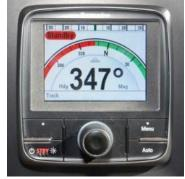
**Bring up rudder indicator** – in the upper part of the RayMarine Autopilot display, by cycling through the screens. Move wheel left/right, then set rudder to neutral position, or as desired.
