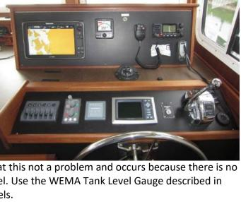
When needed, stop the engine by pressing and holding the soft rubber, black Start/Stop button on the throttle/shifter base until the engine shuts down, then turn the ignition key to OFF.
