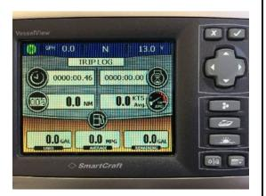
The "Critical Fuel" alarm may sound – press the "X" key at the top right to silence. Note that this not a problem and occurs because there is no link between the VesselView and the fuel tank level sensor. Use the WEMA Tank Level Gauge described above to obtain tank levels.
