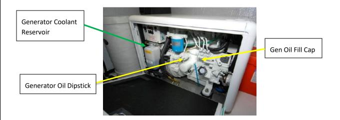
Visually Check the interior of the generator compartment for any leaks or drips. The generator has a diesel engine requiring the same care as the main engine. Open the rectangular panel on the INBOARD SIDE of the generator to inspect.
