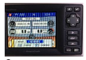
highlight "Trip Log". Press the symbol to select. Press the symbol again to bring up the Reset
