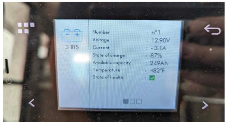
The Victron Cerbo GX display also shows battery voltage, capacity and an estimated draw down time, as well as which systems are contributing power and using power.
