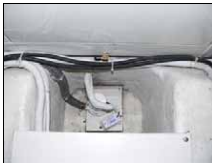
Midships forward is the 17kw Onan Forward midships bilge well with bilge generator; this view with the starboard pump and float switch access door open with the yellow dipstick on left and oil fill pipe center.
