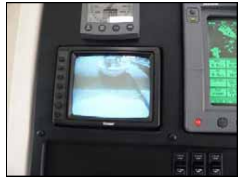
The closed circuit TV. The photograph of the image was blurred due to the TV's "scan" rate: the image is actually quite good!
