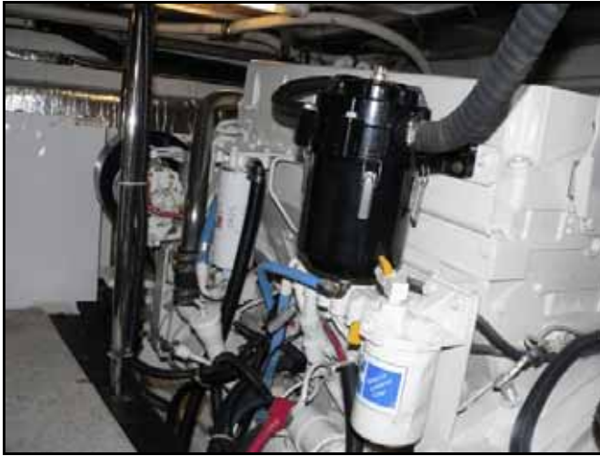
The starboard main engine, looking forward, Onan cabinet on left. The oil filler and dipstick are easily accessible low on the engine beneath to forward blue fuel line under the fuel filter.
