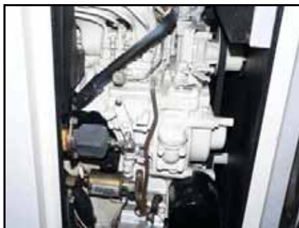
Midships forward is the 17kw Onan Forward midships bilge well with bilge generator; this view with the starboard pump and float switch access door open with the yellow dipstick on left and oil fill pipe center.
