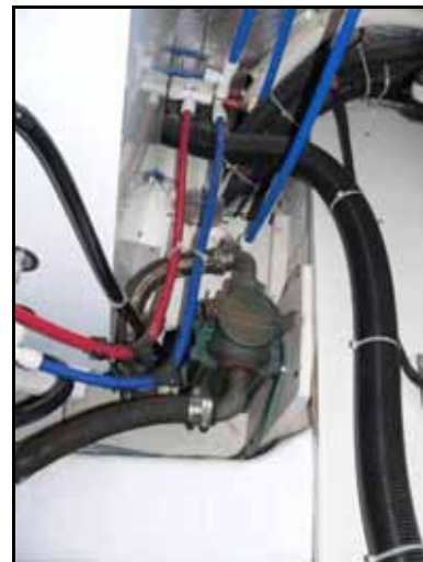
The genset sea strainer, with its through-hull right next to it, forward in the engine room.
