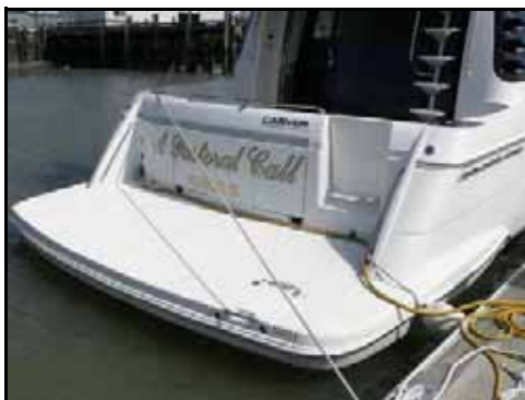
The huge swim step, with shore power cable in place. Beneath one section of the swim step is a sturdy ladder; storage compartments in the transom hold lines, etc.
