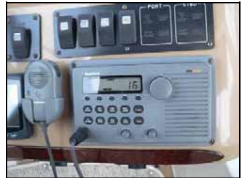
The VHF radios are to the right of each helm station. This is the pilothouse unit.
