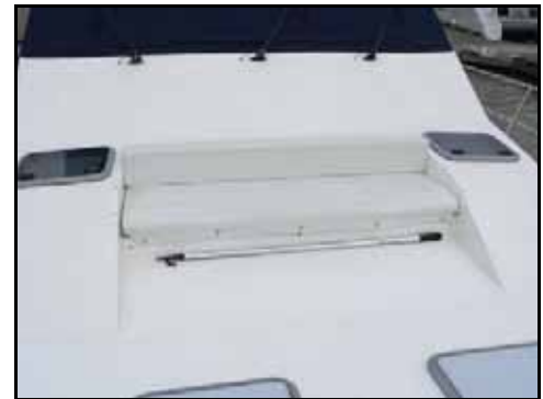
The bow deck lounge. Hatches each side are deck equipment storage cabinets.
