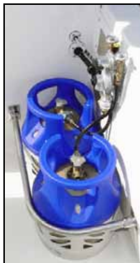
The galley propane tanks are mounted on the aft side of the flybridge settee
