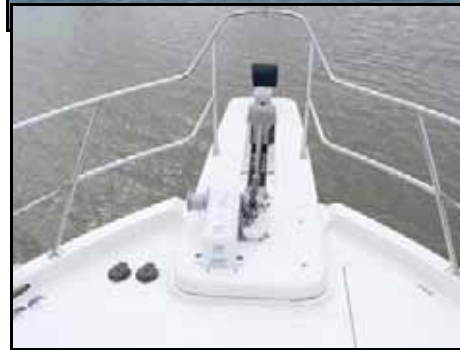
(Above) The bow pulpit with windlass and foot switches. Bow hatch to right with washdown. (Right) The wide walk-around side deck.
