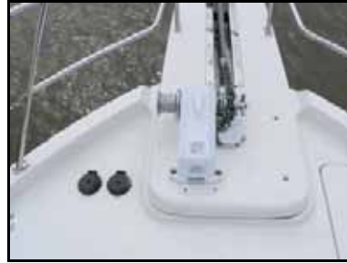
Anchor Windlass; Foot switches to left.
