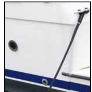
Diesel furnace exhaust is the large outlet in the white hull topsides.
