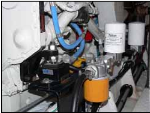
The starboard engine dipstick and oil fill is the yellow T-handle just above the filter.
