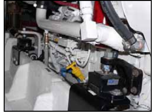
The port engine dipstick and oil fill is the yellow T-handle just aft of the forward engine mount.
