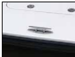
One of the retractable cleats in the "up" position.
