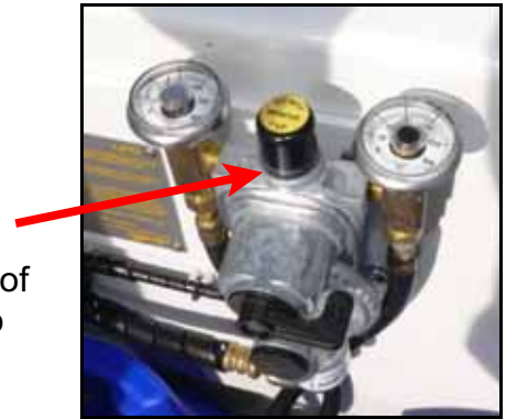
(Above) The propane tanks, control above. (Below) The control. Arrow points to indicator band.
