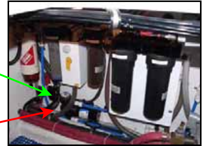
(Above) To starboard in the forward engine room compartment. (Below) To port are filters and controls (green) for the watermaker and (red) water pump.
