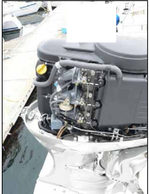
Motor with cover removed. The dipstick is near the bottom flange for the cover, while the oil fill is the yellow cap.
