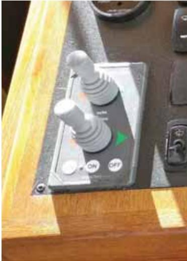
**The thrusters should be used in short bursts and only to rotate the vessel. They should not be used to maneuver the vessel, for example, for finding the ‘right’ spot to drop anchor, to pick up a buoy or to maneuver through a marina. Over-use of the thrusters will quickly deplete the thruster batteries and leave you without their valuable assistance.**
