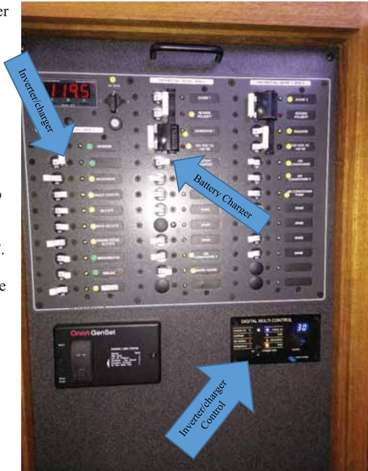
There are systems in place on KINGFISHER to protect against a damaging draw-down of the batteries. These systems include breakers, Automatic Charging Relays (ACRs) and, finally, various fuses.
