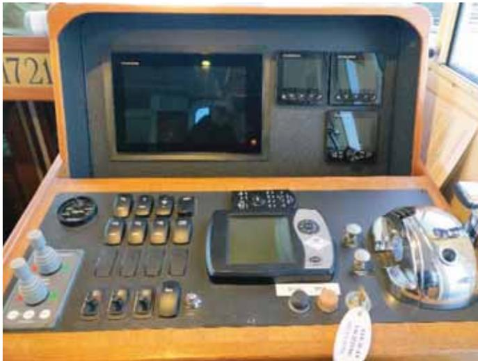
In the photo at left, the chart plotter is the large display on the left. The autopilot (Furuno NAVpilot-71 IC) is located at the lower right. Above the autopilot are two multi-function displays. The one to the right is wind speed/direction and the MFD to the left displays speed, course and depth.
