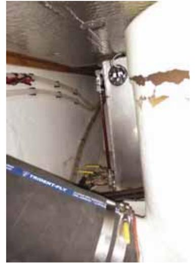
*Starboard Fuel Tank and Sight Tube*
