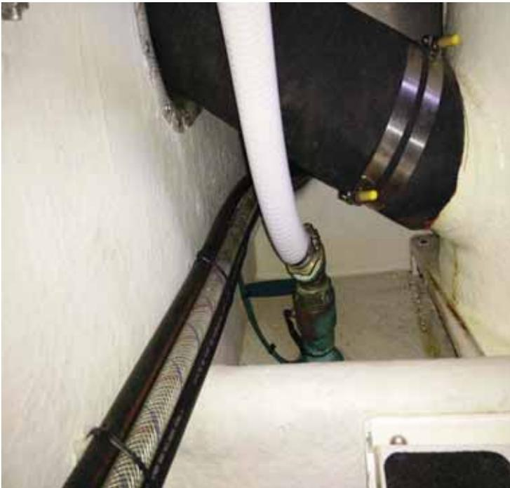
If dumping overboard (into the crystal clean waters of the Salish Sea) is necessary, follow this procedure. **First, and critically important, you must open the macerator seacock to allow waste to exit the macerator into the sea.**
