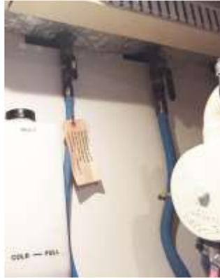
Main fuel tank valves in front of each engine. Turn off for all fuel filter changes.
