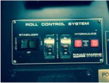
The stabilizer is enabled when the 'electronics' breaker is turned on. Press the switch to 'Center' to activate the system. It may take 5 minutes for the system to warm up to operating temperature. Switch to 'ON' to engage the stabilizer.
