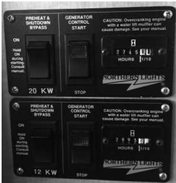
IF THE GENERATOR SHUTS DOWN: Check for a closed thru hull valve, low oil, low coolant, or plugged sea strainer. If problems persist, call SJYC.
