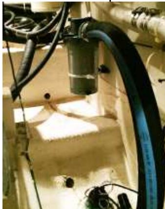
Raw water supply through hull
