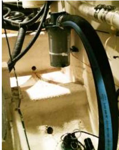
Port Engine Strainer with through-hull valve closed. Heat Pump Strainer forward of port engine.
