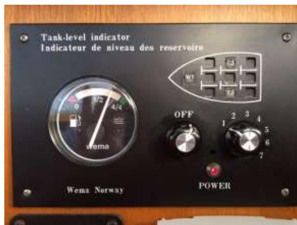
**Note:** the Wema gauge works only when the nautical instrument breaker #40 is on.
