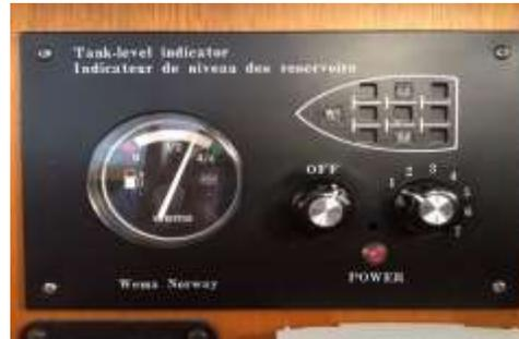
**Note:** the Wema gauge works only when the nautical instrument breaker #40 is on.
