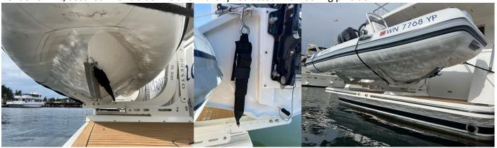
Lift and tender in intermediate position, full extended position, and lowered with tender in water. Outboard raised 30 degrees to prevent damage to swim step when tender moved over the swim step.
