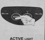
WILL FLASH WHEN ACTIVE BUTTON IS PRESSED AT INACTIVE STATION **CONTROL HANDLES** must be in an appropriate handle position at station taking control in order for transfer to be completed (see chart below). When handles are in an appropriate handle position for transfer, the ACTIVE light will begin to flash quickly.
