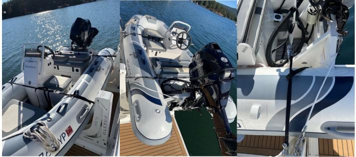
Primary 2-inch ratcheting tie downs at bow & transom attached to the lift via holes in the support arms. Tender on lift, secured with tie downs and lift fully retracted with locking pins down.
