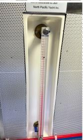
Make sure you do not overflow!! Fuel spillage is very serious and can result in substantial fines. Pay Attention and be careful. Repeat for the other tank.
