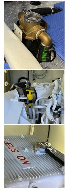
those "soapy" looking tide and eddy lines in the water and they should be avoided. When eelgrass gets sucked into the engine cooling water intake, it collects in the raw water strainer, and impairs the flow of water needed to cool the engine. To clear eelgrass from the raw water strainer:
