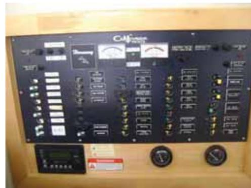
If no AC power source is available, the left hand gauge in top center will read "0 volts." The gauge to the right of this indicates DC battery voltage. A multi-position rotary switch selects which battery set is sensed by the meter: Port = House Main batteries; Aux = Genset battery; Stbd = Engine Start Battery. **Normal voltages: 12.2 – 14.0 volts DC.**
