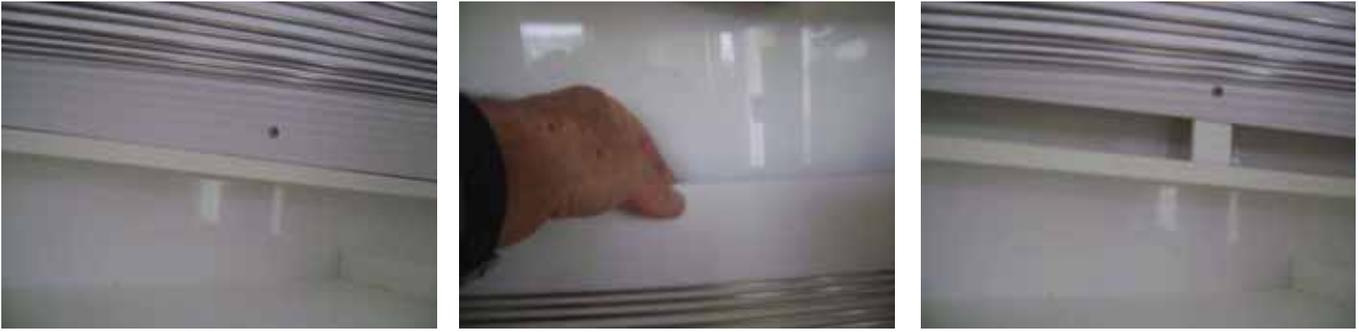
So we've found that in cooler temps or when access to the frig is infrequent, keep the panel in the lower position. And in warmer periods of time, raise the panel to the upper position will more effectively cool the frig and keep things frozen in the freezer.
