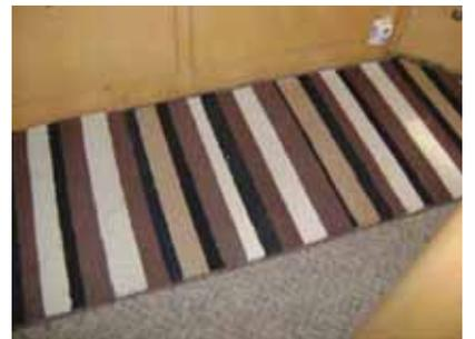
Access is gained by pulling up the carpeting at the foot of the berth in the forward stateroom (start at the starboard end and gently fold it back towards the center walkway), then find the large area of carpet padding that is cut out and separate with a finger hole. Pull up that section of the pad and then pull the removable hatch panel in the subfloor. You now have access to the vacu-flush pumps and just to starboard of this hatch is the through hull for the macerator (normally closed).
