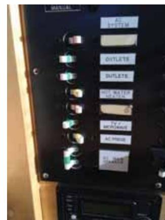
\*If the house batteries have had significant use without recharging, the inverter (in charging mode) can draw up to 1,000 watts. Watch loads carefully and allow the Magnum charger to come up to full current before adding other loads while on shore power, especially the water heater. This can take a minute or two. Watch amp meter when adding load. Multiply amps by 10 to approximate the load in watts from the charger. **Add up the power you are using; be sure it's under the limit!**
