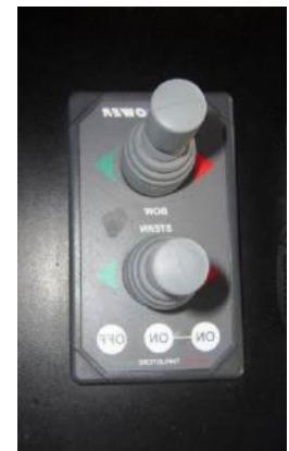
**Use the thrusters in short bursts of 3 - 5 seconds to prevent overheating.** If the thrusters are used continuously for more than 2 minutes they may overheat. It can take 10-15 minutes for the thrusters thermal protection fuse to reset after overheating.
