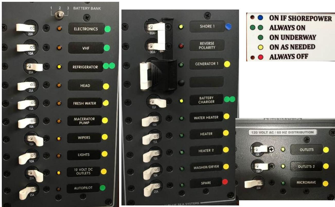
When not connected to shore power or when using the generator as an A/C source, the batteries are providing all power. Therefore, monitor the use of onboard electricity carefully with your volt meter located on the DC Panel, and turn off electrical devices that are not needed. Note: switches controlling the batteries are located next to the starboard side helm seat.
