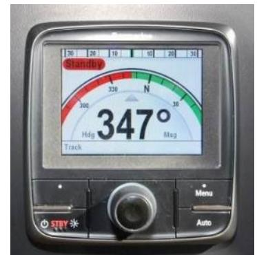
**Bring up rudder indicator** – in the upper part of the RayMarine Autopilot display, by cycling through the screens. Move wheel left/right, then set rudder to neutral position, or as desired.
