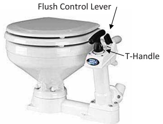
The Flush Control lever should always be on Shut (→) and the T-handle should be locked (white arrow on T-handle pointing to locked icon) except when flushing to prevent flooding the boat in case of valve failure. Move the lever to Open (←) to bring water in and out, then back to Shut (→) to empty the bowl. If it gets hard to flush, try “oil and vinegar”. SJS staff puts vinegar and vegetable oil in the head cabinet.
