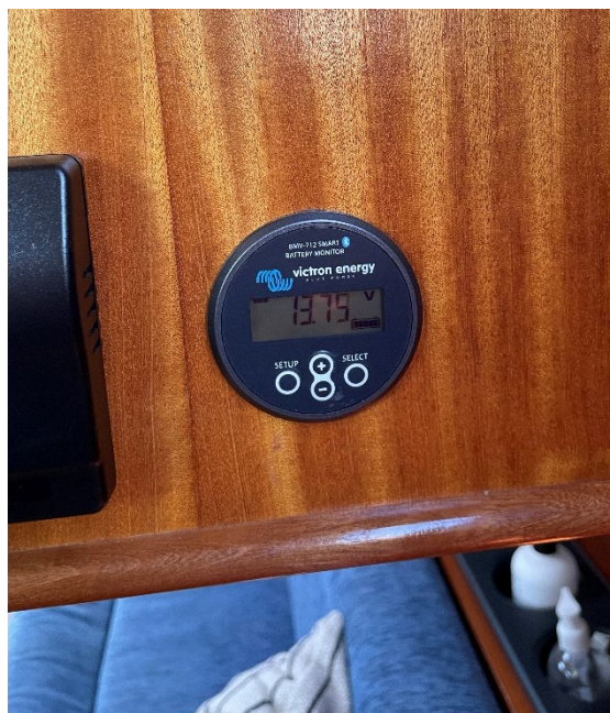
House battery on/off switch (leave on) located under forward berth, just forward of the battery. House battery monitor located above forward end of nav station. Charge battery no later than 13.0v or 20% state of charge.
