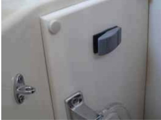
After pushing the “sump pump” breaker to “on” at the electrical panel, the pump is controlled by the grey switch, shown above, mounted on the wall by the head sink.
