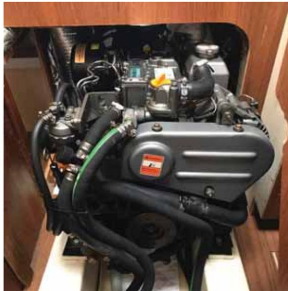
The oil dipstick is on the left side of the engine. The engine is not known to use oil; nevertheless, a spare quart is stored with spare parts. Mechanics check the oil levels weekly.
