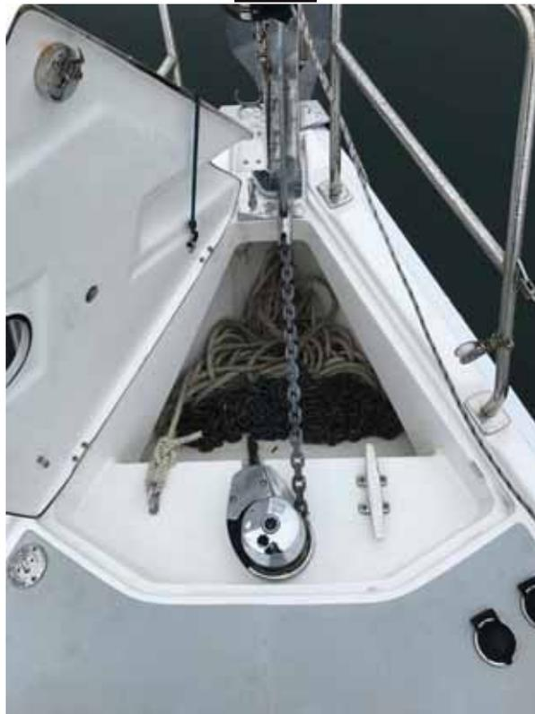
Main anchor – 35 lbs. Lewmar Delta (plow) mounted on the bow, with 150' 5/16" chain marked with 10' yellow paint at 100', and 5' yellow paint at 150'. 150' 9/16" line.
