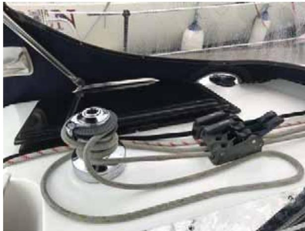
An alternate approach (which we prefer) is to have one crewmember go up to the mast and use the winch there to furl in the sail. It is faster and requires way fewer turns on the winch. Be sure to have another crewmember hold the outhaul and keep the boat just off the wind so it furls up tight. No need to hold onto the continuous furling line.
