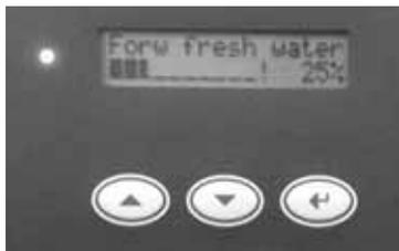
At the top left is an LCD display that you can page through using the “up/down” buttons, to monitor battery charge, water tank, and waste tank status.
