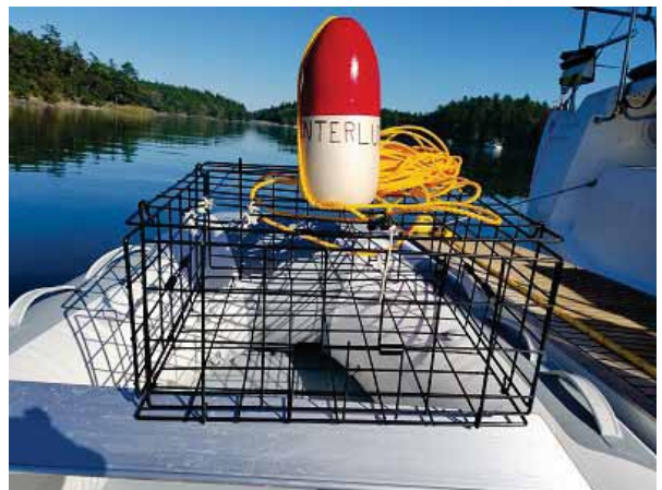
Collapsible Crab Pot - Top Attaches to Side Panels with U-shaped Retaining Clips
