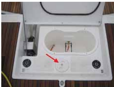
Propane Locker with Emergency Tiller Access (arrow), Diesel Fuel Port (right) and Aft Water Tank Port (Left)
