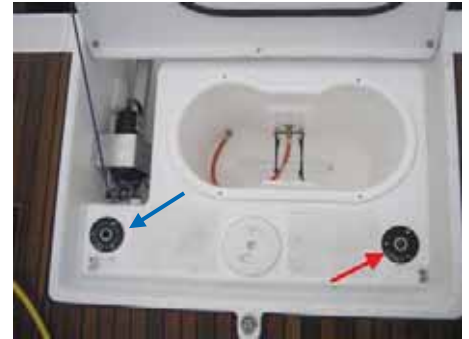
Fuel Tank Fill Port in Propane Locker (red arrow); Aft Water Tank Fill Port (blue arrow)
