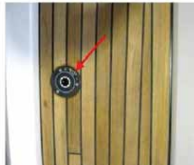
Forward Water Tank Fill Port - Port Deck
