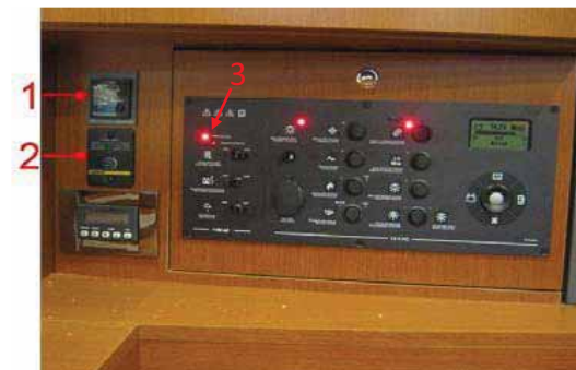
Inverter Controls: Voltmeter (1), ON/OFF Switch (2) AC Shore Power Light (3)
