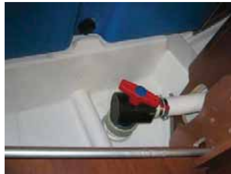
Forward Head Overboard Discharge Valve – Located in Forward Cabin in Storage Compartment under Bunk
