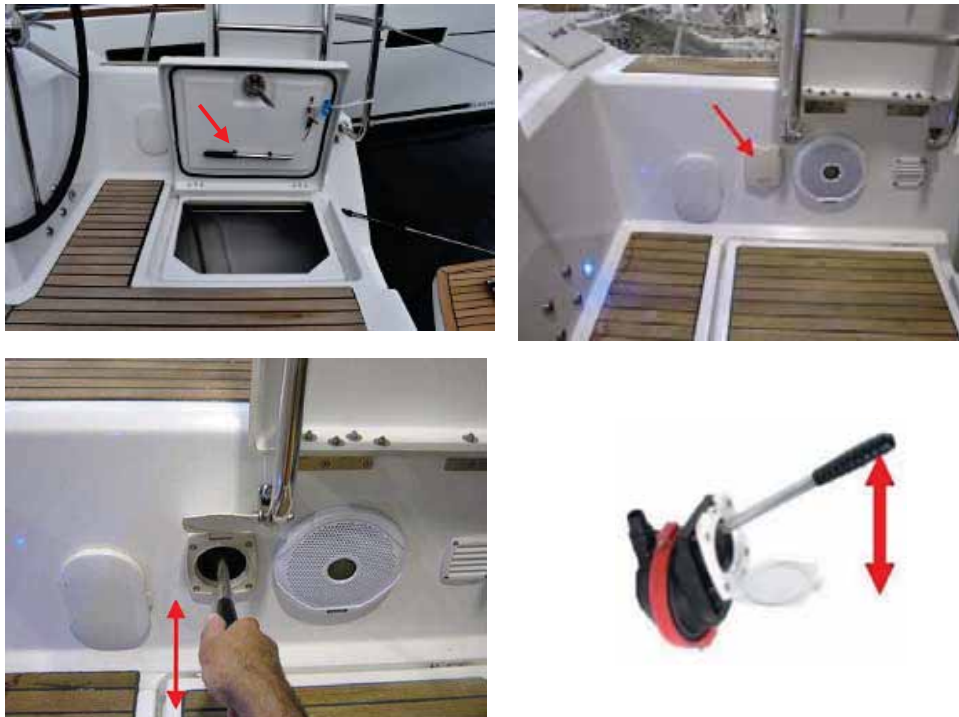
Operating the Manual Bilge Pump (handle clipped under starboard cockpit locker hatch)
