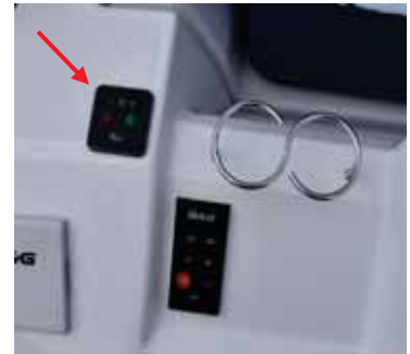
Bow Thruster Controls (red arrow)
