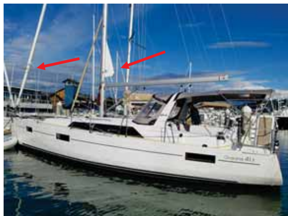
Furled Mainsail & Foresail - Note Mainsail Clew Exposed and One Wrap of Jib Sheets around Genoa
