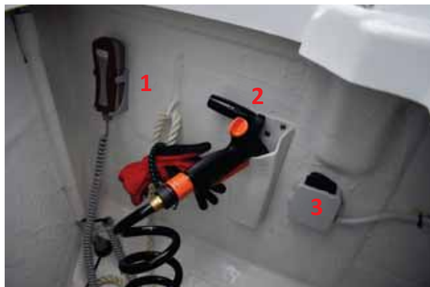
Anchor Locker with Windlass Controller (1), Wash-down Hose (2) and Wash-down Pump Switch (3)
