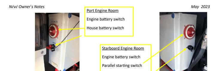
The parallel switch on the starboard engine compartment panel is the emergency crossover should you ever need it. Again, it should normally remain in the vertical/off (facing down) position.
