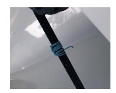
• Press the up button on the controls (port side of cockpit) until the blue threads on the lift line approach the winch drum near the ceiling (see picture to right).
