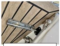
Port tailgate bolt in locked position.
