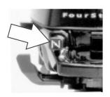
9. Check for a steady stream of water flowing out of the cooling water exit hole. IMPORTANT: If no water is coming out of the water pump indicator hole, stop the engine and check cooling water intake for obstruction.
