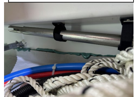
Emergency Tiller in the port lazarette as viewed to starboard and aft Clipped to Transom horizontally.
