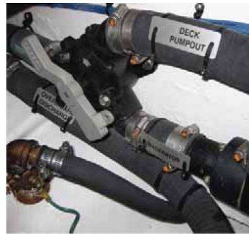
*A view of the Y-valve controlling movement of waste from the holding tank with flow directed to the deck pumpout*
