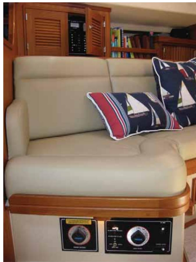
*Battery switches below the port settee and the electrical panel above*
