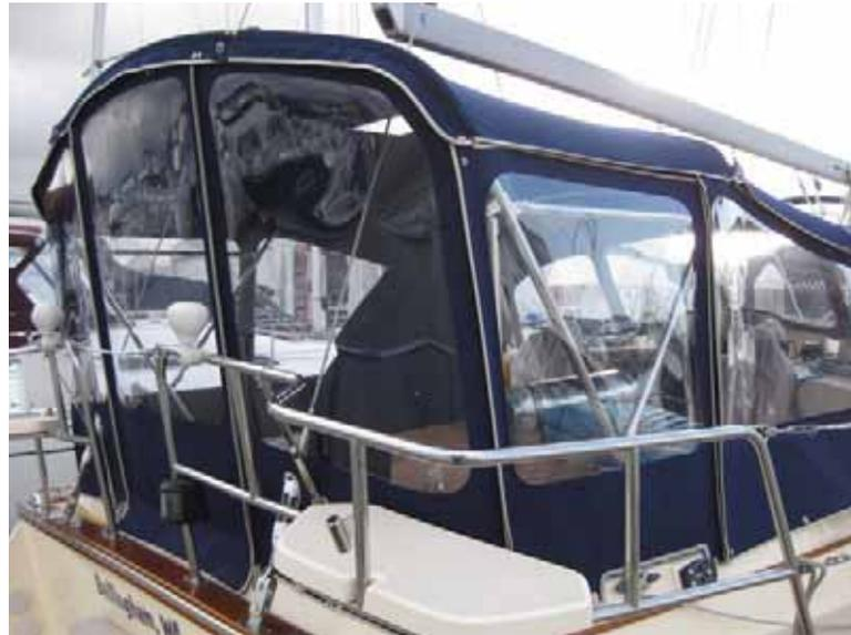
*A view of the cockpit enclosure with all side and rear panels in place*
