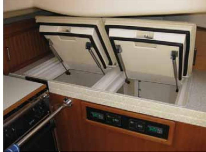
*Refrigerator/freezer compartment lids open and showing the digital control panel*
