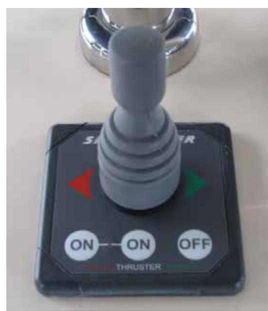
*Puffin's bow thruster control joystick on the port side of the binnacle*
