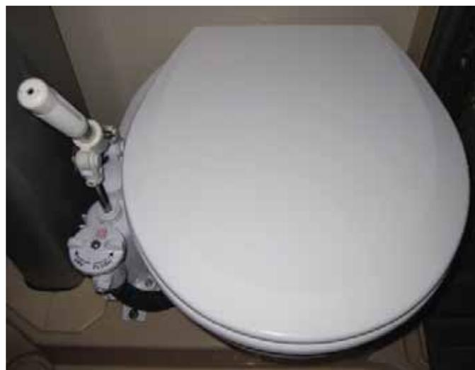
*A view of the marine toilet in Puffin's head showing the pump handle and two-position valve at left*
