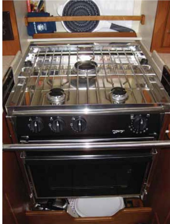
*The Force 10 propane stove and oven showing the three burner controls (left) and the oven control (right)*
