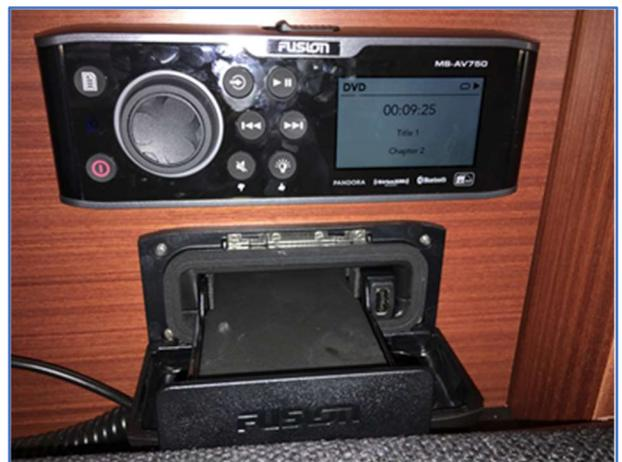
**Media (smartphone) Player** – Open the face of the lower Fusion player (the latch is on top, pivot face down), connect smartphone with USB cable (not provided).
