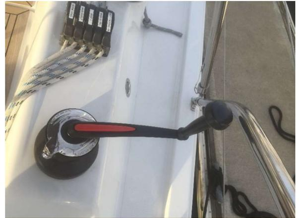
We have two different length winch handles on board. There is one longer, more powerful winch handle (shown) and two shorter winch handles. The longer handle is handy for raising the main, however as seen in the picture, it comes very close to the bimini frame, so you do have to watch your fingers in the pinch point. Please be careful if you use the longer winch handle to raise the main.
