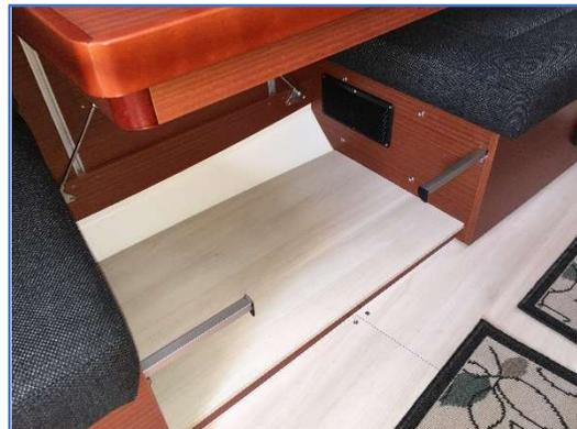
3. Fill the nav table space with the folding backrest cushion located at the aft end of the aft nav station settee. The folding backrest cushion on the forward end can be used as a backrest if you wish to use the entire length as additional seating.
