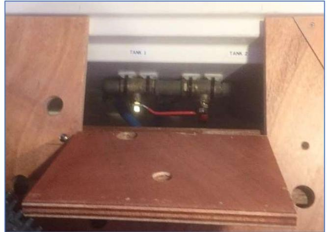
Water Tank Valves under starboard side of V-berth cushion.
