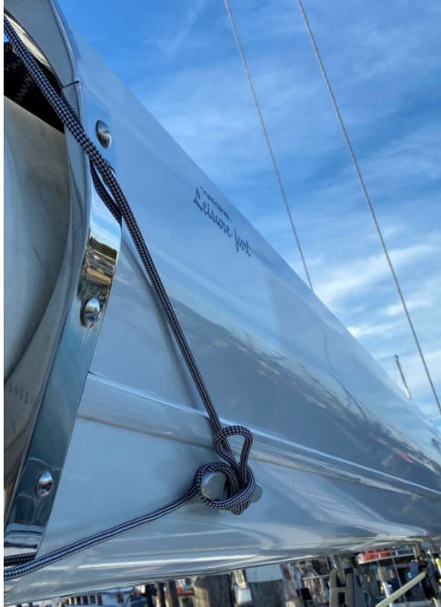
Cleat for the sail cover. There is a line, and cleat, on each side of the boom.
