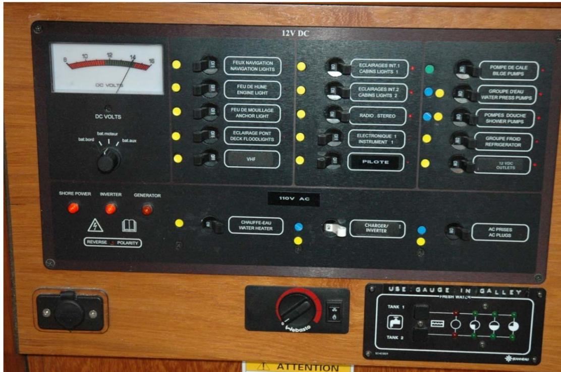
Most switches at the panel board at the Navigation Station to port in the main salon are self-explanatory, but some circuits are unique.
