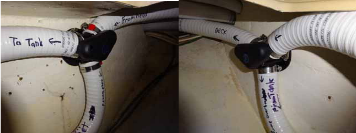
Toilet to Tank or Overboard (Aft Y-Valve) Tank to Deck Fitting or Overboard (Forward Y-Valve)
