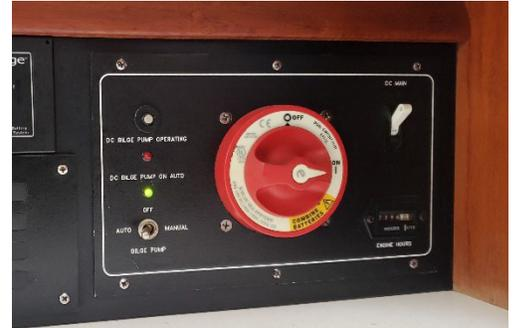
You may occasionally hear the pump operate due to condensation and water from the shaft seal accumulating in the bilge. If you hear the bilge pump running a lot, you need to check the bilge for leaks. One source to check for a leak is the lid on the seagrass trap for the sea water engine cooling water, located under the bed in the aft stateroom. It can leak if not seated properly. Th
