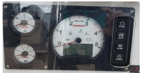
operating correctly. **(NEVER turn off the Power with the engine running as it may blow the diodes on the alternator and it will cease to charge the batteries; push the Stop button first.)**
