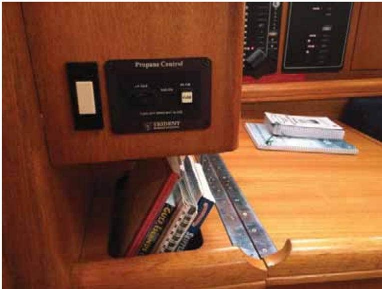
Cabin light switch (left) and propane solenoid switch. Propane LPG switch is on the electric control panel.
