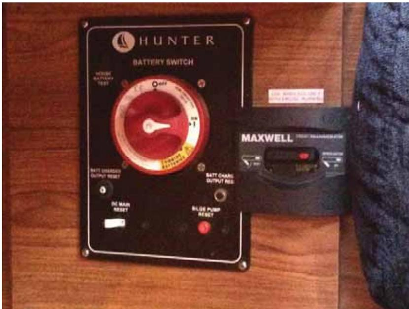
(The circuit breaker for the Windlass is under the Nav table at the right in the picture above. On the left is the switch to combine batteries for emergency engine start as well as reset switches)
