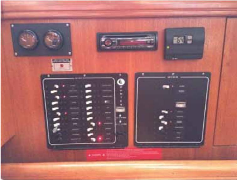
(Clockwise from upper left -*Tank indicators* for water, fuel, and red holding tank full indicator; *stereo*, *heater thermostat* with on/off switch, *AC panel* for shore power; *DC panel* for battery power.)
