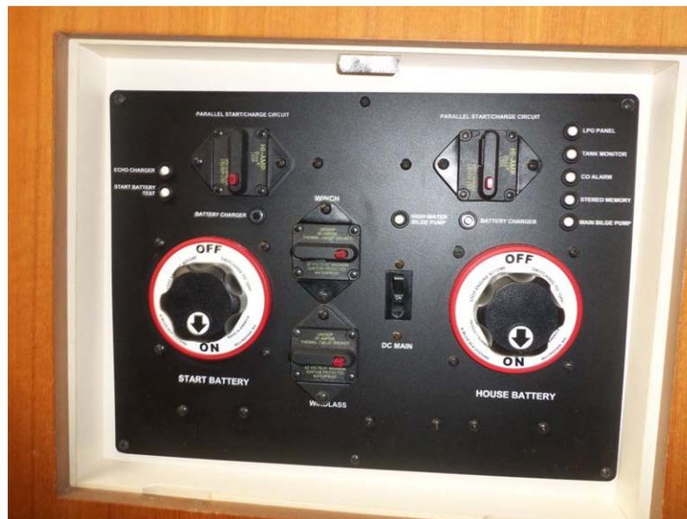
Battery voltage can be checked on the electrical panel. The starting battery is labeled “start” and the house battery is “house”, a toggle switch changes the display to reflect what you are monitoring. You should try not to discharge below 11.5 volts before re-charging the batteries by (1) running the diesel or (2) plugging into shore power. The charger is below the seat in the living room next to the kitchen.
