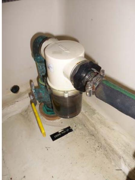
*If upon restarting the engine overheats again, check the seal between the strainer, the rubber gasket, and the container. If the strainer is drawing air, it won't draw water. If needed, open and then retighten the lid on the strainer...and check to make sure the rubber gasket is in place in the lid (and not lying in the bilge.)*
