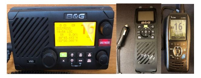
From Left to Right: Main Ship Radio, Wireless Remote, Handheld VHF/GPS
