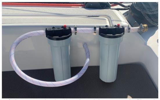
For freshest water, use the onboard hoses along with this contraption when filling tanks.
