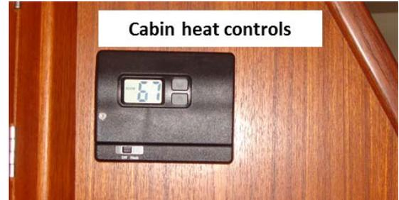
*The heater is large for this size boat (we use the boat mostly during the off season when temperatures are lower). To avoid the heater cycling on and off rapidly in warmer weather, keep all the heater vents (forward cabin, main cabin, aft cabin open) and the doors to the aft cabin, head, and forward cabin open, so that the heater has to heat the entire boat.*
