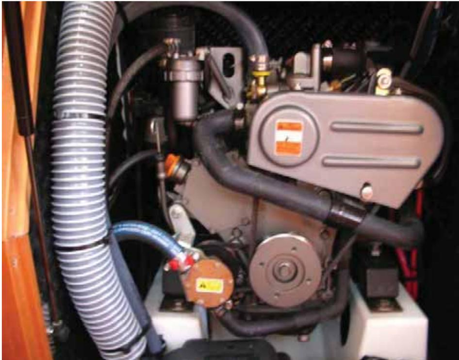
The **coolant level** is visible in the plastic reservoir at the rear of the engine on the port side.
