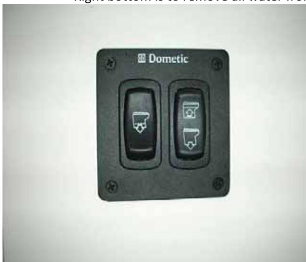
Because this system uses fresh water and you only have 77 gallons, be judicious in your full flushing. For example, if no solids are involved, then just removing the liquid is most efficient (right bottom). The water pressure breaker must be ON to operate the toilet. The master breaker for the toilet is inside the panel under the Nav table. It's inside on the aft side of the panel opening.
