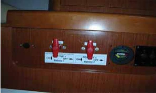
Red Start Battery Switch: The engine will not start without this being ON (vertical position)
