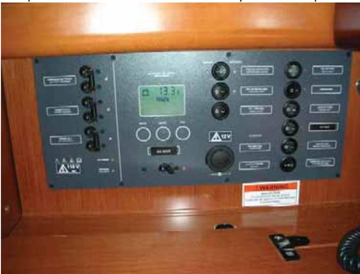
**AC Panel:** The left side of the electrical panel is the AC side and has three double pole switches [from top to bottom]: Battery Charger, Water Heater, and AC Outlets. Below that are two lights which indicate AC power is present, and a Reverse Polarity light which indicates that something is wrong with your shore power source and you should disconnect until the problem is corrected. **DC Panel:** The center and right side of the panel is the DC side.
