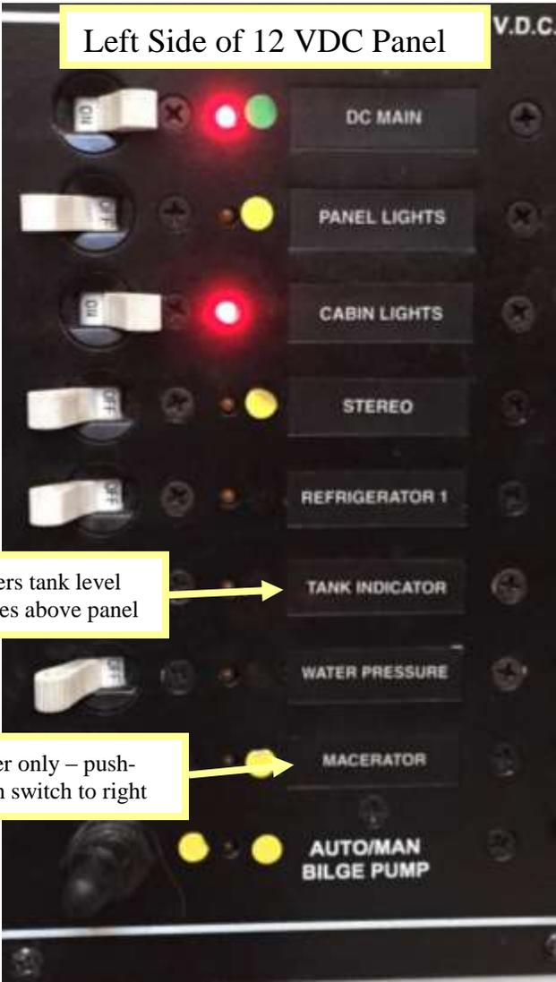
Powers tank level gauges above panel
